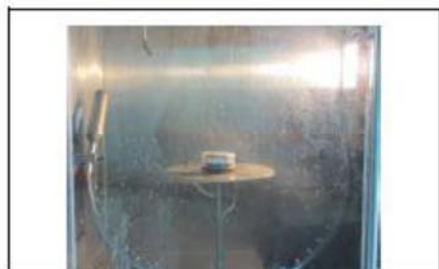
C12-B During the Rain Test
